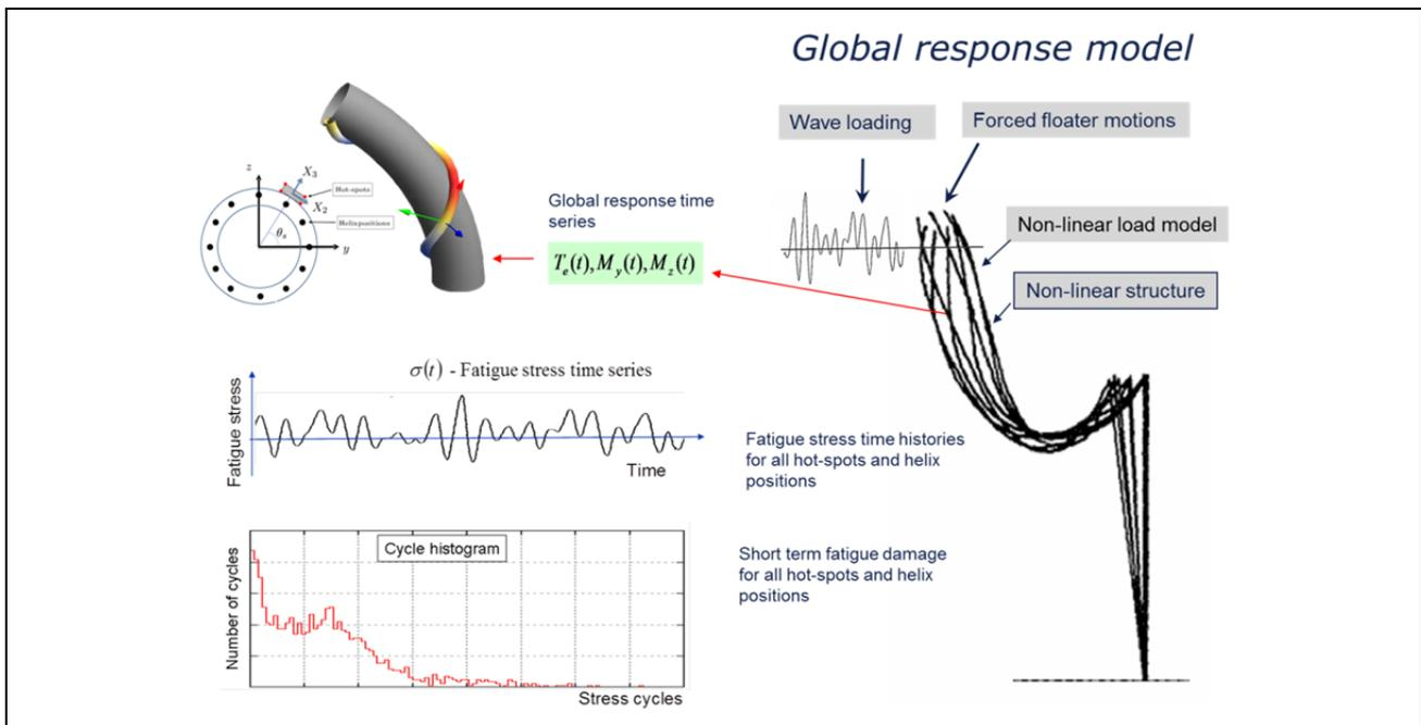
The output from the analysis is short-term fatigue damage and stress cycle distributions to be applied in subsequent long-term fatigue analysis.
