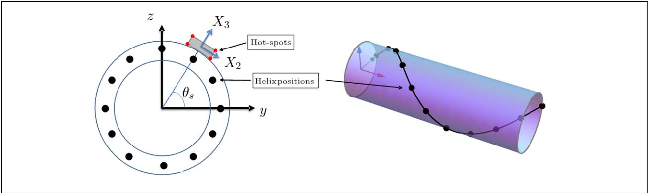
The main challenge is hence to establish an overall manageable computational scheme to establish fatigue life estimates with sufficient confidence. A computationally efficient cross-sectional analysis strategy is hence a vital part of the overall fatigue analysis approach. DNV GL has developed a dedicated computer program named **Helica** to address these design and analysis challenges, /3/ and /4/. The main capabilities are:
