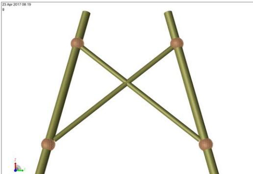
**Two legs, two braces, four tubular joints**
