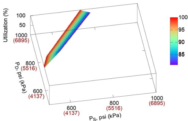
**Figure 9** - Percent utilization as a function of suction (PS) and discharge (PD) pressures at a flow of 200 mmcf/d (5.66 Mm3/d) for compressor RC\_fixed\_s\_var\_cl\_min\_power
