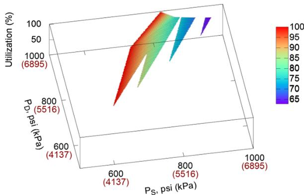
**Figure 3** - Percent utilization as a function of suction (PS) and discharge (PD) pressures for a flow of 300 mmcf/d (8.50 Mm3/d) allowing continuous clearance
