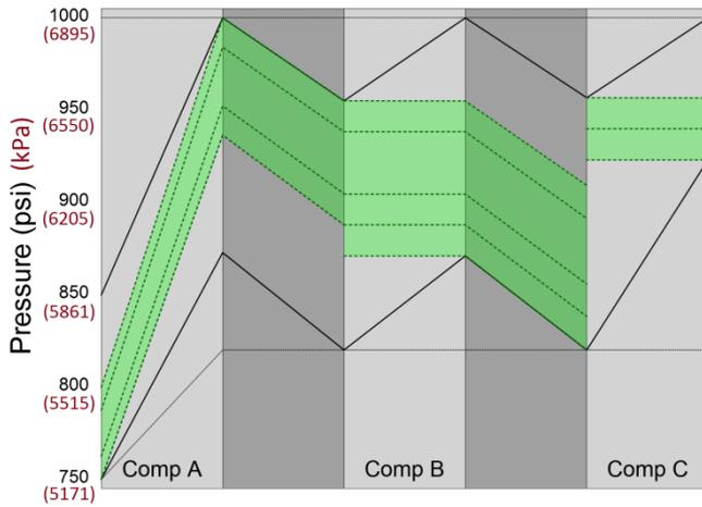
**Figure 10** - Feasibility chart for a pipeline flow of 230 mmcf/d (6.51 Mm<sup>3</sup>/d). Feasible pipeline operation is not possible since the bypass states from compressor B do not intersect with bypass states on compressor C
