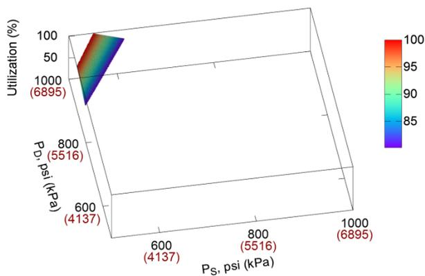
**Figure 11** - Percent utilization as a function of suction (PS) and discharge (PD) pressures at a flow of 100 mmcf/d (2.83 Mm<sup>3</sup>/d) for compressor RC\_fixed\_s\_var\_cl\_min\_power
