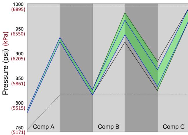
**Figure 13** - Feasibility chart for a pipeline flow of 335 mmcf/d (9.49 Mm<sup>3</sup>/d). All three compressors are compressing
