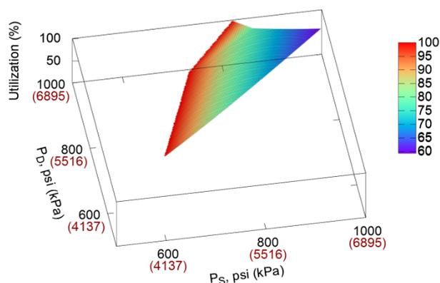
**Figure 4** - Percent utilization as a function of suction (PS) and discharge (PD) pressures for a flow of 300 mmcf/d (8.50 Mm<sup>3</sup>/d) allowing continuous clearance and allowing the speed to vary between 250 and 300 rpm
