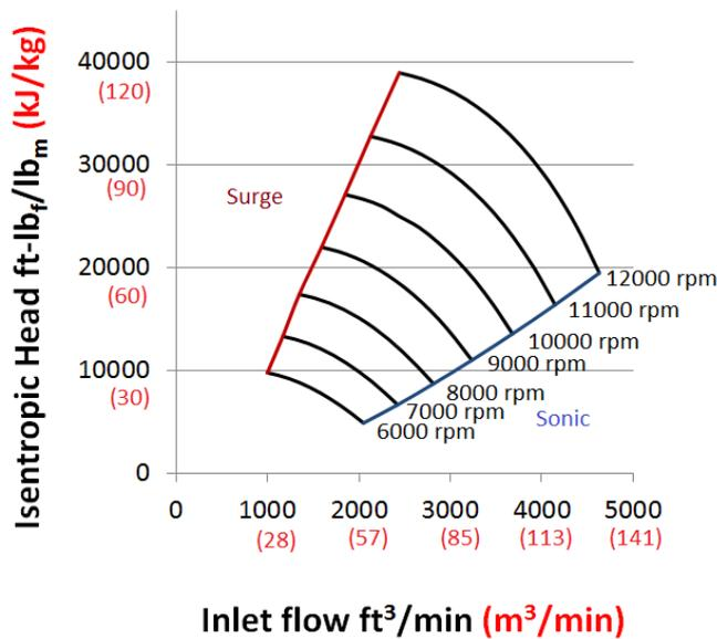
**Figure 13** - Head flow map for compressor CC
