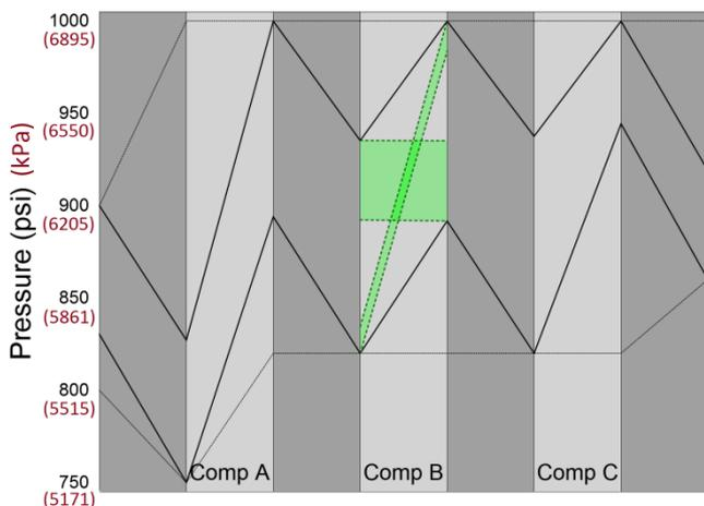
**Figure 7** - Pictorial representation of the feasibility table for compressor B at a flow of 275 mmcf/d (7.79 Mm<sup>3</sup>/d); the horizontal green box represents feasible compressor bypassed states, while the sloped green section represents feasible compression states
