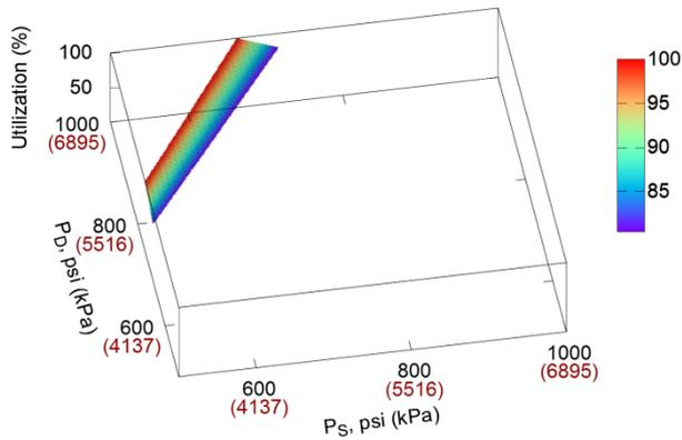
**Figure 10** - Percent utilization as a function of suction (PS) and discharge (PD) pressures at a flow of 150 mmcf/d (4.25 Mm<sup>3</sup>/d) for compressor RC\_fixed\_s\_var\_cl\_min\_power; calculations were performed over pressures ranging from 500 psig (3447 kPa) to 1000 psig (6895 kPa)
