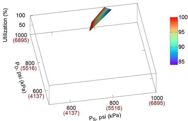
**Figure 6** - Percent utilization as a function of suction (PS) and discharge (PD) pressures at a flow of 350 mmcf/d (9.91 Mm<sup>3</sup>/d) for compressor RC\_fixed\_s\_var\_cl\_min\_power
