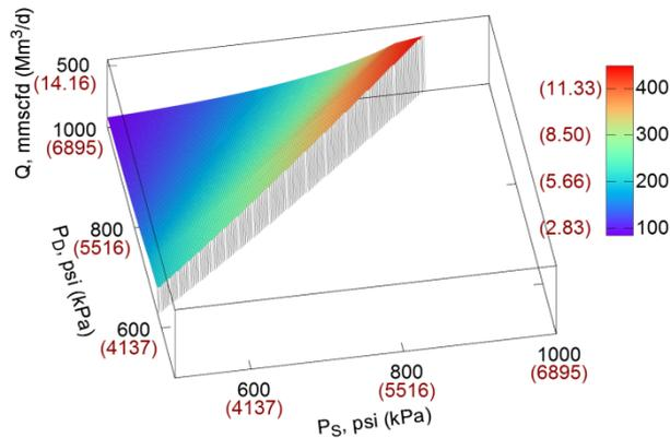
**Figure 5** - Capacity as a function of suction (PS) and discharge (PD) pressures for compressor RC\_fixed\_s\_var\_cl\_min\_power
