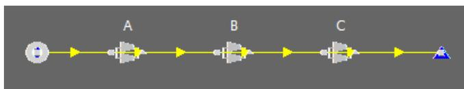
**Figure 25** - Fictitious pipeline containing 3 compressor stations each separated by 75 miles (121 km) of 28 inch (711 mm) pipeline; all pipes are 75 miles (121 km) long
