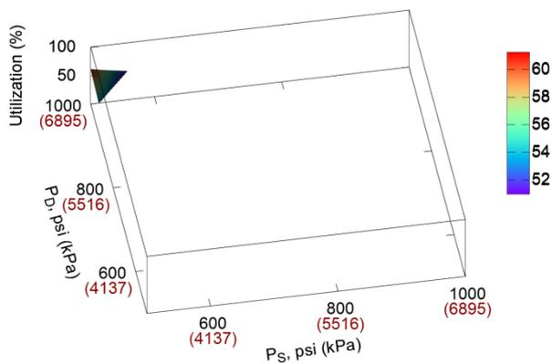
**Figure 18** - Centrifugal compressor percent utilization at a flow of 100 mmcf/d (2.83 Mm<sup>3</sup>/d) as a function of suction (PS) and discharge (PD) pressures
