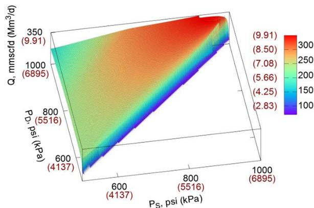
**Figure 3** - Centrifugal compressor capacity ( $Q$ ) with no minimum power and sonic operation allowed
