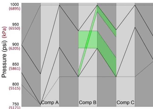
**Figure 30** - Pictorial representation of the feasibility table for compressor B at a flow of 275 mmcf/d (7.79 Mm<sup>3</sup>/d); the feasible region corresponding to the discharge of compressor B is extended through the downstream pipes to the suction of compressor C
