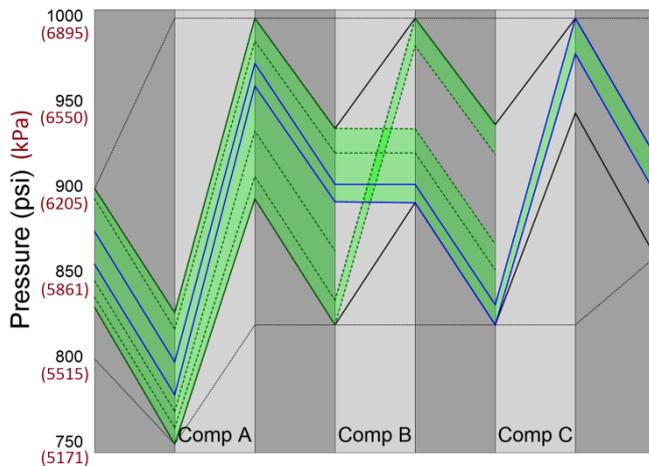
**Figure 32** - Pictorial representation of the feasibility table for all compressors at a flow of 275 mmcf/d (7.79 Mm3/d); the feasible pipeline operating region is indicated by the area between the blue lines
