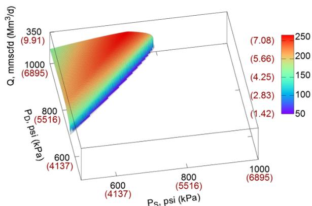
**Figure 15** - Centrifugal compressor capacity as a function of suction (PS) and discharge (PD) pressures; minimum power is set to 60% of maximum power
