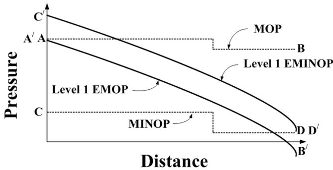
Figure 22 - Infeasible level 1 pressure envelopes
