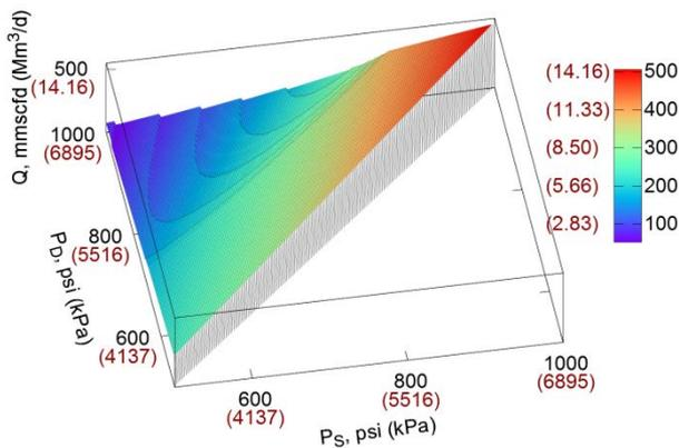
**Figure 1** - Capacity (Q) of compressor RC\_fixed\_s\_fixed\_cl as a function of suction (P<sub>s</sub>) and discharge (P<sub>d</sub>) pressures
