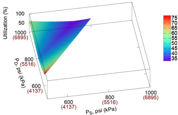
**Figure 2** - Centrifugal compressor percent utilization at a flow of 100 mmcf/d (2.83 Mm<sup>3</sup>/d) as a function of suction ( $P_S$ ) and discharge ( $P_D$ ) pressures with no minimum power applied
