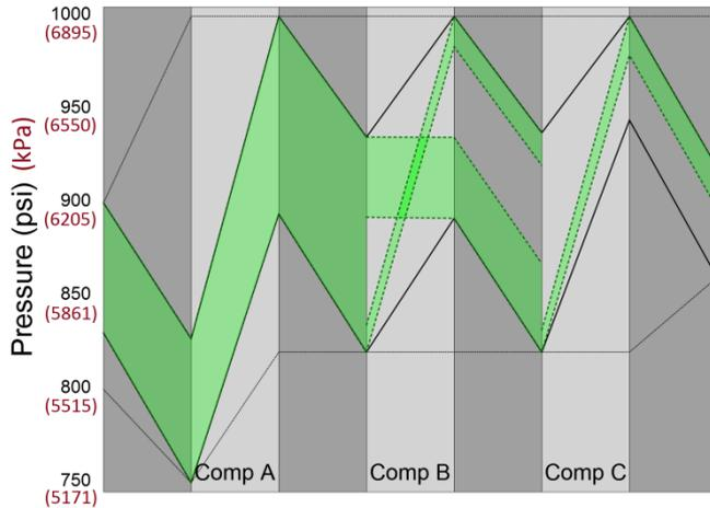
**Figure 31** - Pictorial representation of the feasibility table for all compressors at a flow of 275 mmcf/d (7.79 Mm3/d)
