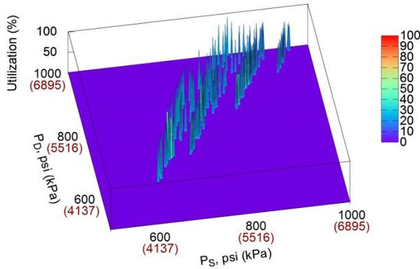
**Figure 2** - Percent utilization as a function of suction (PS) and discharge (PD) pressures for a flow of 300 mmcf/d (8.50 Mm3/d)
