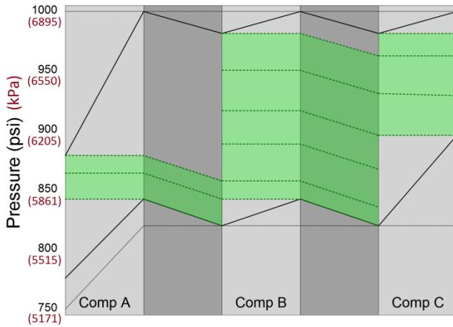
**Figure 8** - Feasibility chart for a pipeline flow of 150 mmcf/d (4.25 Mm<sup>3</sup>/d). The pipeline cannot be operated since there is no connection between feasible regions through the entire pipeline. The frictional pressure loss through the pipes is too large to meet the minimum delivery pressure and compression is not possible due to minimum power requirements.
