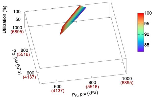
**Figure 7** - Percent utilization as a function of suction (PS) and discharge (PD) pressures at a flow of 300 mmcf/d (8.50 Mm3/d) for compressor RC\_fixed\_s\_var\_cl\_min\_power
