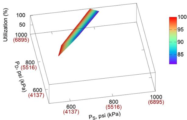
**Figure 8** - Percent utilization as a function of suction (PS) and discharge (PD) pressures at a flow of 250 mmcf/d (7.08 Mm3/d) for compressor RC\_fixed\_s\_var\_cl\_min\_power
