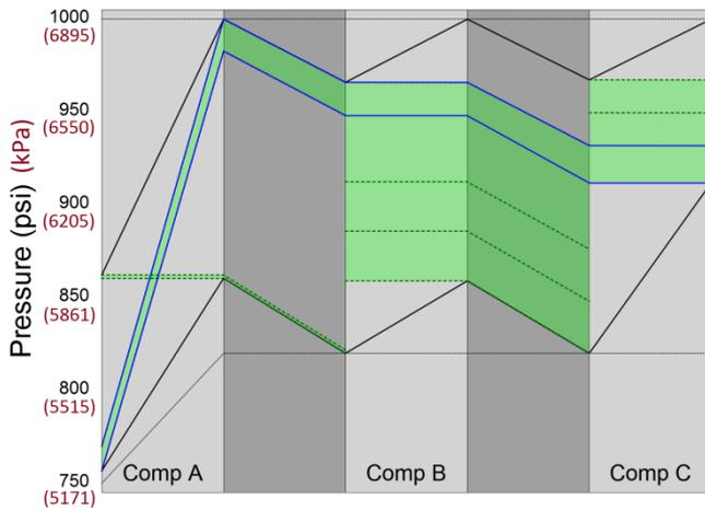
**Figure 9** - Feasibility chart for a pipeline flow of 200 mmcf/d (5.66 Mm<sup>3</sup>/d). Compressor A is compressing while compressors B and C are bypassed
