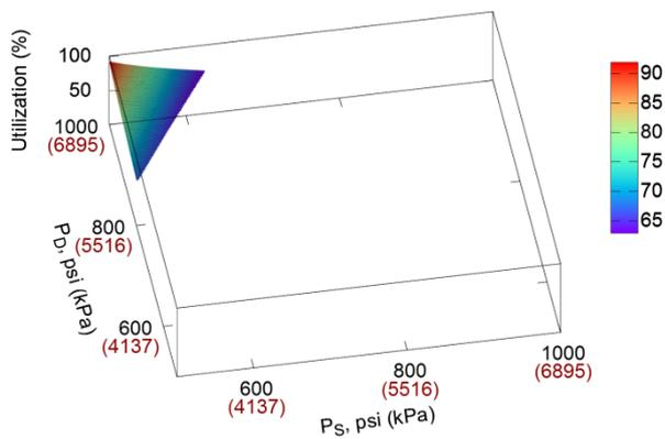
**Figure 17** - Centrifugal compressor percent utilization at a flow of 150 mmcf/d (4.25 Mm<sup>3</sup>/d) as a function of suction (PS) and discharge (PD) pressures; minimum power is set to 60% of maximum power
