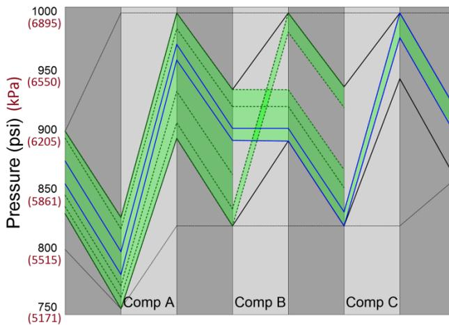
**Figure 11** - Feasibility chart for a pipeline flow of 275 mmcf/d (7.79 Mm<sup>3</sup>/d). Feasible operation consists of bypassing compressor B and compressing through compressors A and C
