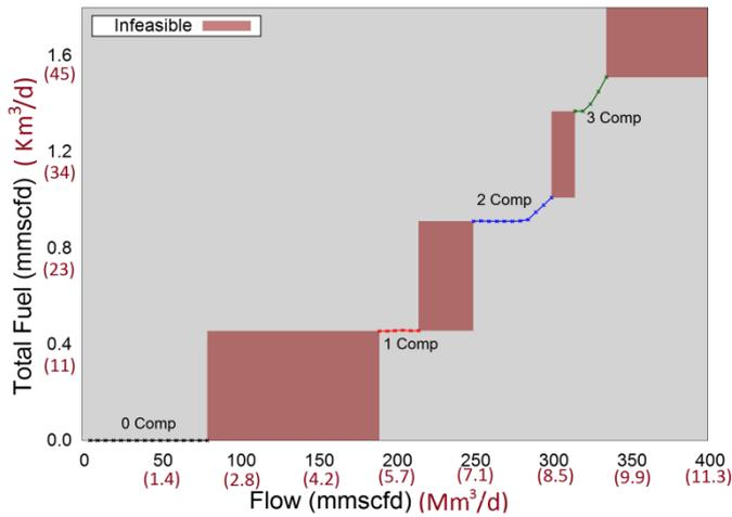
**Figure 33** - Pipeline fuel usage as flows are varied from 0 to 400. The red regions represent flows with no possible feasible pipeline operation
