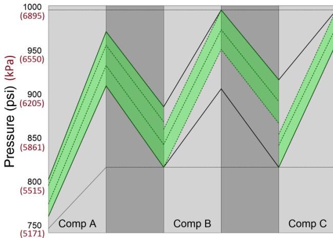
**Figure 12** - Feasibility chart for a pipeline flow of 310 mmcf/d (8.79 Mm<sup>3</sup>/d). Feasible pipeline operation is not possible since gas enters compressor C at too high a pressure
