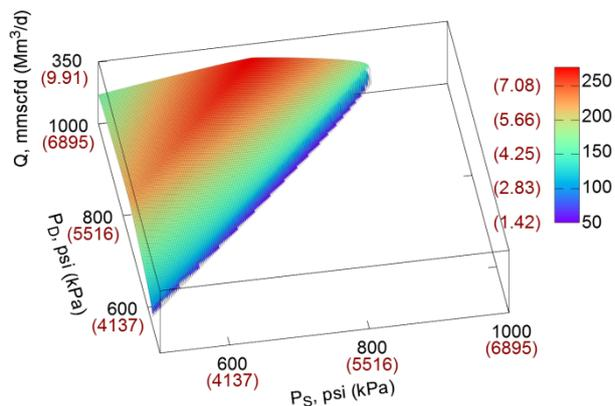
**Figure 14** - Centrifugal compressor capacity as a function of suction (PS) and discharge (PD) pressures
