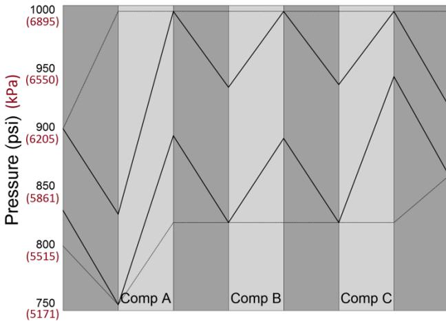
**Figure 5** - Maximum and minimum pressure envelopes for a flow of 275 mmcf/d (7.79 Mm<sup>3</sup>/d)
