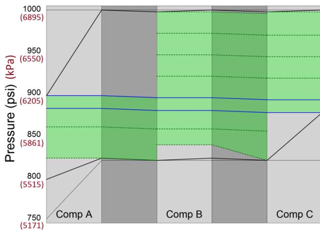
**Figure 34** - Feasibility chart for a pipeline flow of 50 mmcf (1.42 Mm<sup>3</sup>/d). The only feasible operating mode is to fully bypass all compressors.
