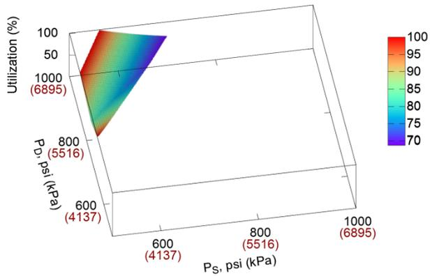
**Figure 16** - Centrifugal compressor percent utilization at a flow of 200 mmcf/d (5.66 Mm<sup>3</sup>/d) as a function of suction (PS) and discharge (PD) pressures; minimum power is set to 60% of maximum power
