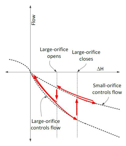
The air-valve constricts the air flow if the head differential across it is large and allows flow through a larger orifice if the head differential across it is small. This causes the air to be released at a slow rate.
