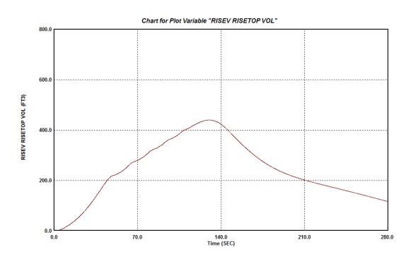
The outflow of air from this air-valve occurs at a slow rate and follows a pattern shown in the figure below.
