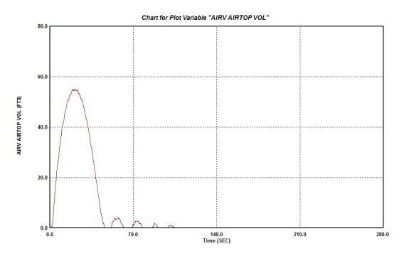
The inflow of air into this air-valve follows a pattern shown in the figure below. As the pressure at the top of the first hill begins to fall, the small-orifice air inlet opens and draws air into the pipeline. As the pressure continues to become more negative, the large-orifice vacuum breaker opens. As the pressure begins to increase, the vacuum breaker closes. However, the small-orifice air inlet/relief valve stays open and gradually expels the trapped air.
