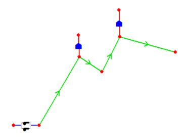
Pump spin down sends a pressure wave through the pipeline. When the pressure at the top of the hills becomes negative, air begins to flow into the air-valves to relieve the negative pressure. When the pressure at the top of the hills returns to positive, air begins to flow out of the air-valves. The amount of air in the air-valves also cushions the pipeline against pressure transients generated during pump spin up.
