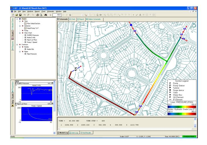
LIQT also provides sophisticated tools for searching through the results and scoping reports to those results. Hydraulic conditionals can be set up that will stop the simulation when a particular hydraulic condition has been met. Also, LIQT can be initialized automatically by generating a steady-state solution or by allowing the user to specify the initial conditions. Vapor cavity formation and collapse can be modeled with LIQT.
