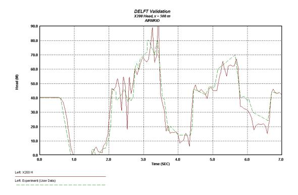
The third validation case is a valve stroking test case. The experimental results are reported in Valve Stroking To Control Transient Flows In Liquid Piping Systems4. Once again, LIQT's results compare well against the experimental results of Propson.
